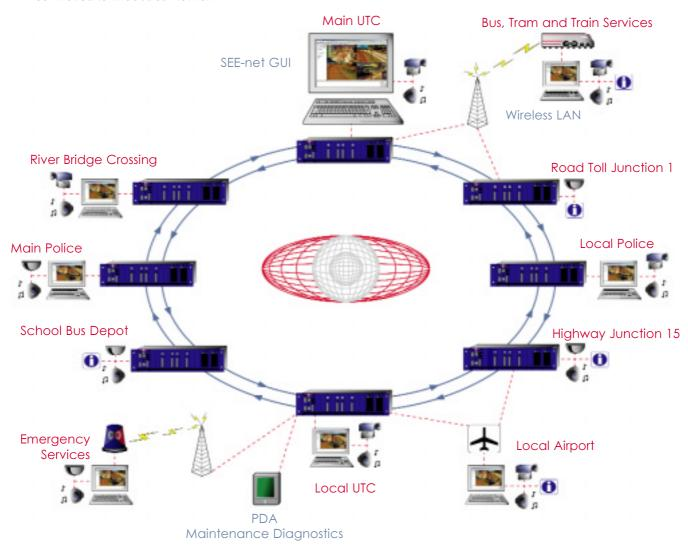
A typical system consists of a core IP network, either as a closed ring (as shown) or as an open solution utilising your existing LAN/WAN. All peripheral devices can be linked across the network via the Codecs as simple point-to-point/multi-point links or managed centrally via COE SEE-net or master third-party GUI.
