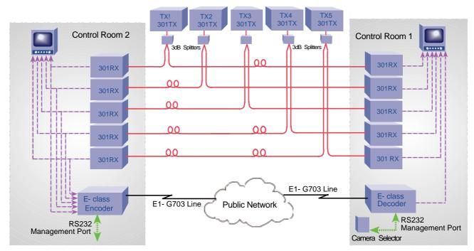
Hence the E-class provides a redundant path which is physically diverse from the main transmission route. The five video inputs are used to select which picture is transported back to the control centre with selection controlled from the VT100 terminal interface.
