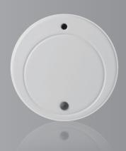
TS-29ZBS is a ZigBee wireless temperature sensor that monitors the temperature of your surrounding environment. Detecting temperature from -10°C to 50°C, it reports temperature condition to the ZigBee gateway at regular intervals, and also sends notification when the temperature fluctuates by +/-2°C.
