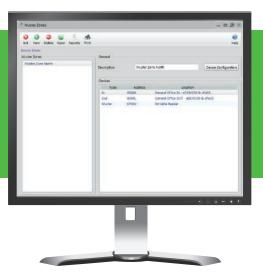
The AC2000 Muster Zones application is used for emergency situations where card holders must congregate in a dedicated 'safe' location. The application can be used both in the evacuation of card holders to a location away from the site (or zone) or when necessary it can be used to enable card holder's to move to a particular safe location within the premises. AC2000 Muster Zones is used in conjunction with the AC2000 Zone Monitoring application.
