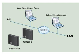
The ACS OnSite control panel can accommodate up to 30 readers. Local Administrator Access is via a Web browser over the Local Area Network (LAN). Remote Access can be set up with the appropriate network configuration, so that the system can be administered from any Web browser with Internet access.
