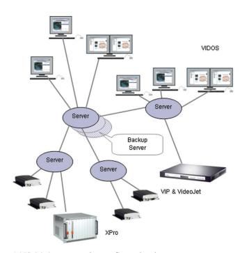
A VIDOS Server can be configured to be master server and/or user server, which has the purpose to provide a single central location for all users and user groups. Both configuration types may be backed-up by other servers configured as backup servers.
