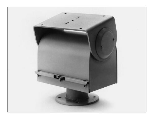
The TC6570PT Series are medium duty pan/tilts for indoor/outdoor operation. These units feature rugged high-torque AC motors, with adjustable worm gear final drives to insure long operational life, as well as drift-free operation. The TC6570PT Series are capable of autorandom scan operation when used with receiver/driver (see Accessories).
