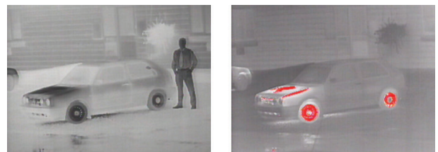
Thermal image in black hot spot mode / Thermal image in ice and fire mode
