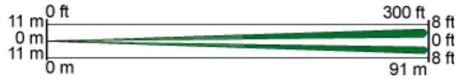
Top View Standard Long Range Coverage: 91 m x 21 m (300 ft x 15 ft). The long range coverage mirror (OA300) is installed.
