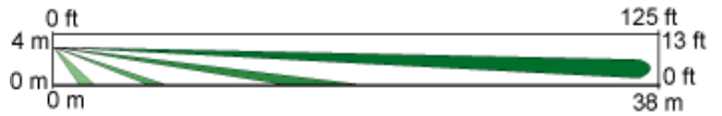
Side View Optional Long Range: 37 m x 8 m (120 ft x 26 ft). The long range coverage mirror (OA300) is installed.
