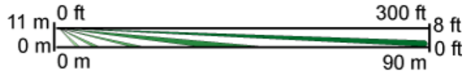
Side View Standard Long Range Coverage: 91 m x 21 m (300 ft x 15 ft). The long range coverage mirror (OA300) is installed.
