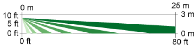
Side View Optional Barrier Coverage: (OMB77) 25 m x 5 m (80 ft x 16 ft)
