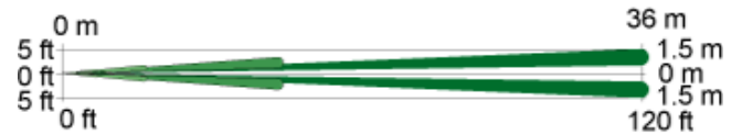
Top View Optional Long Range Coverage: (OMLR77) 40 m x 3 m (120 ft x 10 ft)
