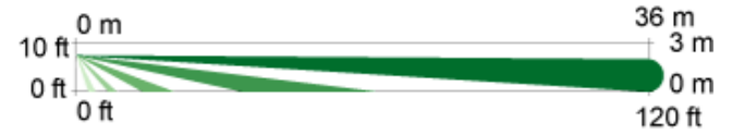
Side View Optional Long Range Coverage: (OMLR77) 40 m x 3 m (120 ft x 10 ft)
