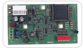
The DX4020 Network Interface Module creates two-way communications over ethernet networks for specific Bosch security control panels. Typical uses include:
