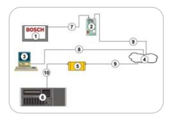
The system overview diagram shows a D6600 NetCom System using a compatible Bosch Security Systems control panel, DX4020 Ethernet Interface Module, D6600 Receiver, and a D6680 Network Adapter.
