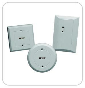
The DS1100i Series are Glass Breakage Detectors which use microprocessor-based Sound Analysis Technology (SAT) to listen for the specific frequencies associated with breaking glass. They can be used to detect breakage of Plate, Tempered, Laminated and Wired glass types. A built-in environmental test feature alerts the installer of false alarm hazards in harsh environments. Several cover designs are available.
