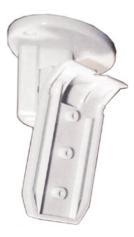
Surface mounts detectors to the ceiling. The vertical pivot range is  $+7^{\circ}$  to  $-16^{\circ}$ ; the horizontal pivot range is  $\pm 45^{\circ}$ . Do not use for pet applications.
