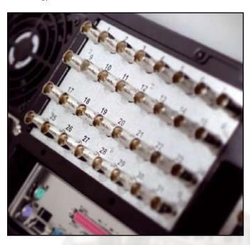
The DVR is fitted with 32 video inputs - 32 analogue or 16 IP and 16 analogue - and a DVD writer to increase the amount of Video sequences that can be copied.
