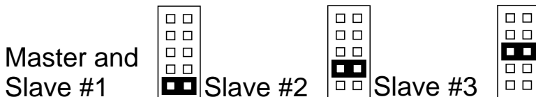
Figure C. Jumper settings in the master and slaves
