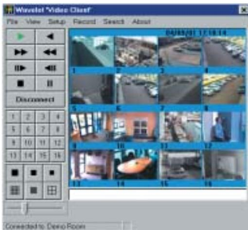
When operated with WaveReader software, the DTL960e can be used to search and view video remotely or directly, either in a live picture mode or playback from the hard drive during which the DTL remains recording.
