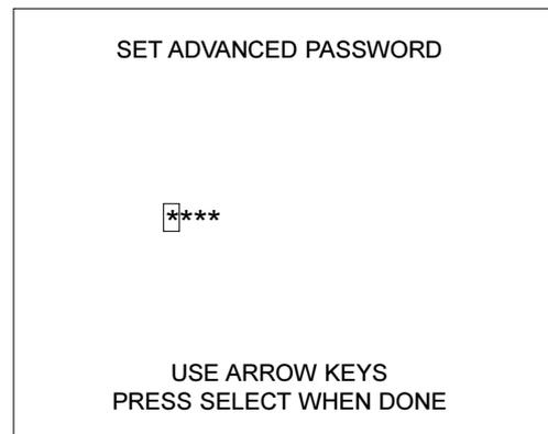
Note that the first digit of the password is selected. To change the password, the up/down arrow keys or joystick are used to select the required number for each of the four digits in the password. An up/down movement of the arrow keys or joystick will cause the selected digit to either increment or decrement. When the digit is correct, use the left/right arrow keys or joystick to move to the next digit of the password. When all four numbers have been set, press the select key.
