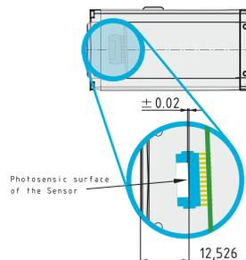
The back focal length on each camera is carefully measured and adjusted by our patented "CSAT" procedure. This guarantees an optimum distance between the lens flange and the sensor and ensures outstanding image quality based on compliance with optics standards.
