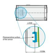
The back focal length on each camera is carefully measured and adjusted by our patented "CSAT" procedure. This guarantees an optimum distance between the lens flange and the sensor and ensures outstanding image quality based on compliance with optics standards.
