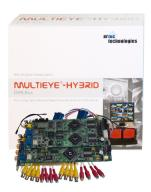
With MULTIEYE®-HYBRID DVR kits, highly professional digital video recorders can be created. MULTIEYE® software supports the simultaneous operation of both analog and digital camera technologies in one system. Up to 32 analog and IP video cameras can be combined and operated with each other in one recorder as desired. Yet the integration of IP cameras is just as simple as setting up analog cameras.
