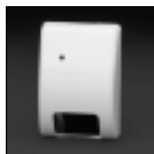
EV 400/MSA EV 400 detector case containing monochrome camera with standard lens and audio
