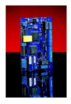
The AIM-2DL has terminations for connection of one or two Wiegand interface readers complete with two LED lines (Red and Green) and a buzzer control line. The interface may be configured to use entry/exit readers at a single door for anti-passback configurations or to use two readers at two separate door with a push-button input for exit (REX). Each reader may also be equipped with a keypad for use in a high security Card plus PIN mode or the user friendly Card or PIN mode.
