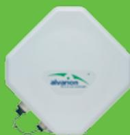
BreezeMAX PRO-S consists of an indoor unit (IDU) and an outdoor unit (ODU) that contains the modem, radio, data processing and management components, as well as an integral high-gain flat antenna with either vertical or horizontal polarization. An ODU with a connector to an external antenna is also available.
