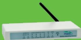
Networking Gateway is the optimal networking solution for both home and small business customers. Featuring an advanced, integrated broadband router with comprehensive IP-sharing and security capabilities, it offers four 10/100 BaseT ports and an 802.11g wireless access point.
