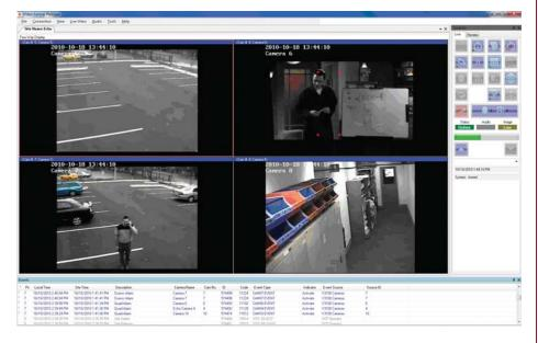
ADPRO VideoCentral Platinum by Xtralis is a multi-site video security management software application specifically designed to monitor video and audio from remote sites fitted with ADPRO video transmission systems.
