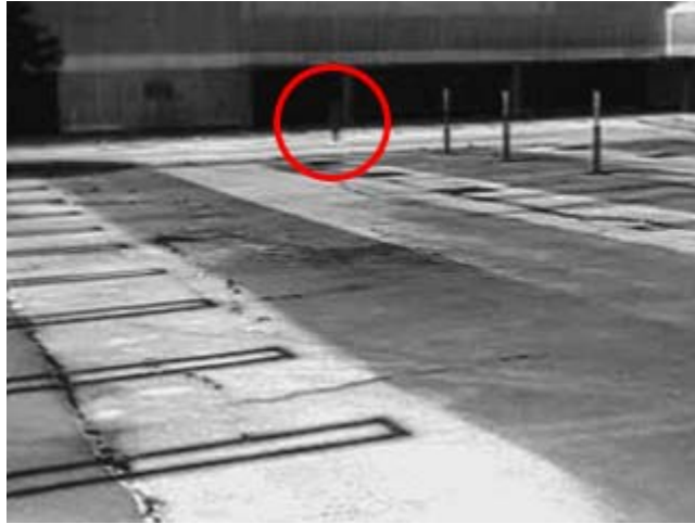
Figure 4: Person Camouflaged by Thermal Crossover
