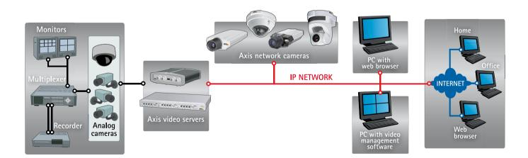
A video server/encoder accommodates one or more analog video channels, image digitizer, image compressor and web server with network interface. Video servers digitize analog video sources and distribute digital images over an IP network, turning an analog camera into a network camera. It is ideal for migrating an existing analog system to a network video solution.
