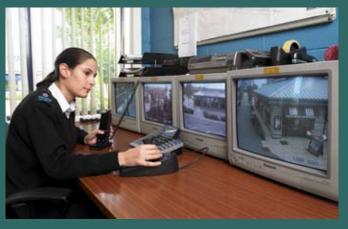
Video playback and review is controlled intuitively via a corresponding WVCU650CJ/B controller that also manages the system's WJ-SX150A camera switching matrix. This type of controller suits a busy Control Room environment.
