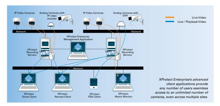
IP video management software Open Software Development Kit (SDK) - Ecosystem Drives Value enables optimal integration with best-of-breed hardware, video analytics and systems. Third Party Applications SDK Interface Decoupling XProtect<sup>™</sup> Enterprise Server Future-proof to your need **Device Drivers** MJPEG / MPEG-4 / MPEG-4 ASP / MxPEG / H.264 IP Cameras IP Encoders DVR / NVR // I/O Devices FREEDOM OF CHOICE
