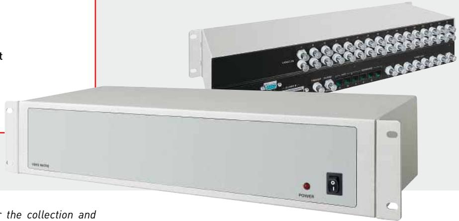
The video matrix SM328B offers a solution for the collection and management of images, capable of switching 32 video inputs to 8 independent outputs and activating 32 different synchronized sequences among several monitors, with day, night or holidays cycles.
