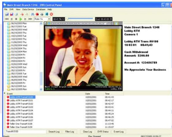
DVR Control Panel software is easy to use. Search for video by time and date, motion event, ATM transaction number, or alarm event. Associated transaction and alarm data are side-bar displayed without obscuring the video, as happens with standard text insertion.
