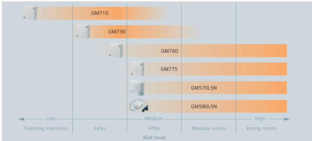
Seismic detectors application range
