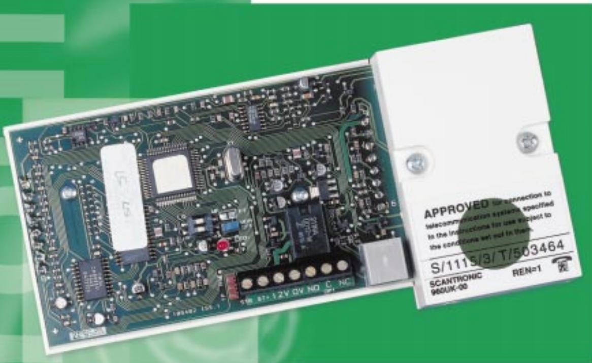
The 960 is a plug-on auto dialling speech/digital communicator unit, designed to be discreetly fitted in a Scantronic, or certain other manufacturer's alarm control panels.
