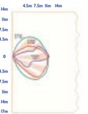
Sample X-band DR0, X-band waveguide and K-band waveguide range adjusted to fit an 11 metre room.
