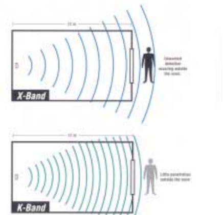
K-band sensors minimize microwave penetration through walls and windows.
