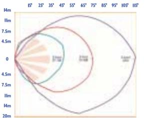
With sensitivity set at 100%, some 11 metre sensors have over 35 metres of microwave range.
