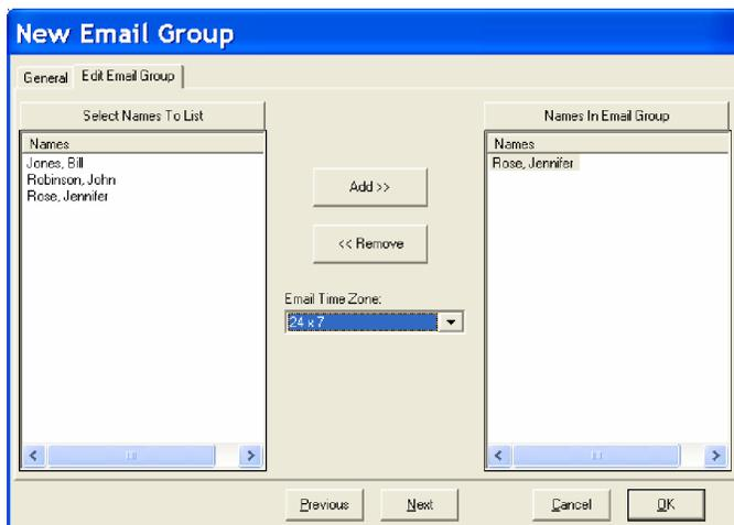
Alarms can also be sent to Cell Phones as Text Messages. Using the Alarm Email Notification feature, an email can be sent to a Cell Phone as a Text Message using the cell phone provider's SMS Gateway. Most Cell Phone providers have a SMS Gateway that will turn an Email into a Text Message and send it to the subscriber's phone.
