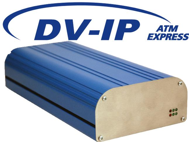
Dedicated Micros DV-IP ATM Express is specifically sized for installation within the confined conditions of an ATM machine or location within a POS area. Capturing and processing transaction data which is then recorded with video footage, the DV-IP ATM Express enables live and post event analysis of transactions via the built in text search engine.
