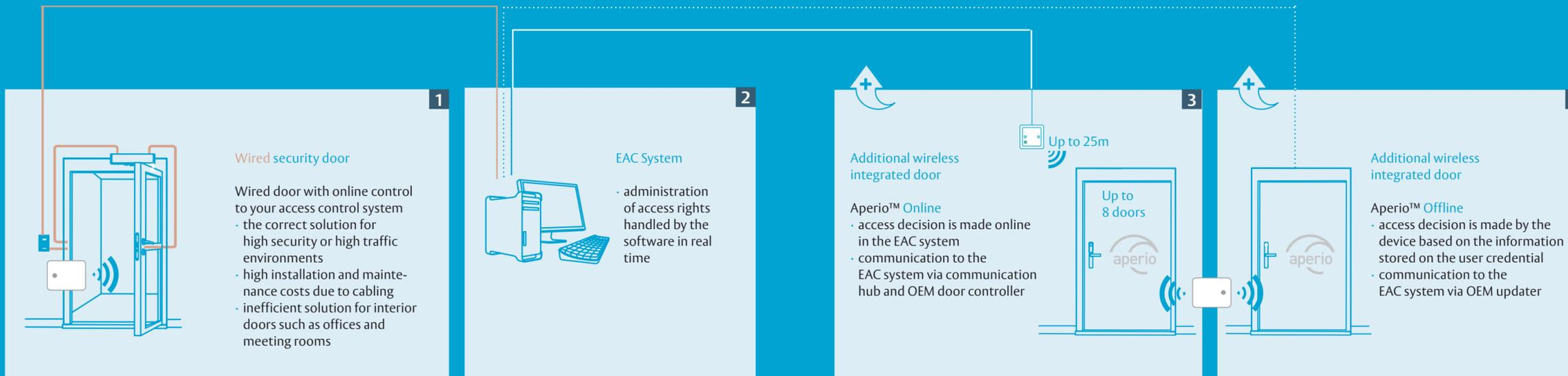
Frequency IEEE 802.15.4 (2,4 GHz) - 128 bit AES encryption
