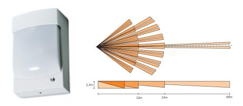
The EV 635 series provides a combined mirror optic with 24m Volumetric, 12m Volumetric and 60m L.R. detection patterns. Using a microprocessor with "4D" processing ensures maximum detection and stability. "Double Check" and "Eye to Eye" features in the EV 640 allow communication between detectors to verify alarms and minimise false alarms. EV 635 – 24m Vol./60m L.R., NC relay
